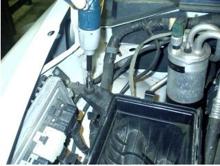
Pull the air filter out of the air box and then remove the 10mm nut at the rear corner of the box.
