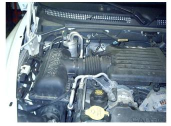
This is what we're starting with – a stock 4.7L intake. Although you won't be touching any electrical connections, its not a bad idea to disconnect the negative battery cable whenever you're working under the hood. You need to reset your computer anyway so that it can re-learn with the new intake in place; if you disconnect it now, enough time will have passed for the computer to be reset by the time you've finished the install.
