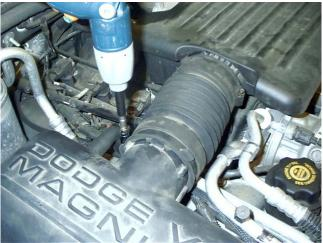
The first step is to loosen the clamps holding the filter box to the plenum. You can either use a screwdriver or a 5/16" hex socket for this. (The socket is easier.)
