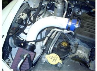
Slide the tube into place on the plenum and the filter into place on the end of the tube.
