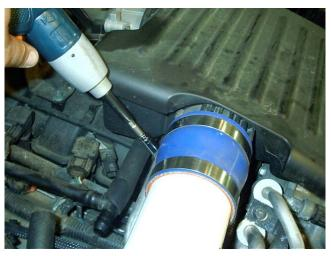
Rotate the tube into the orientation you would like, and then tighten down the band clamp on the plenum side. Be careful here; the band clamp is a high torque style, so you run the risk of cracking the plenum. Just tighten it enough so that it is secure. If you can tug on the intake and it doesn't slip, it probably won't come off on its own either.
