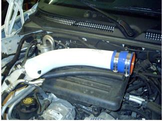
Next, place the silicone connector on the end of the tube which does not have the plastic PCV elbow in it. Set the clamps in place also, but don't tighten them down just yet.
