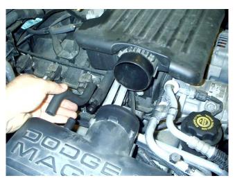
After removing the flex coupling, remove the rubber PCV (Positive Crankcase Ventilation) hose as shown.
