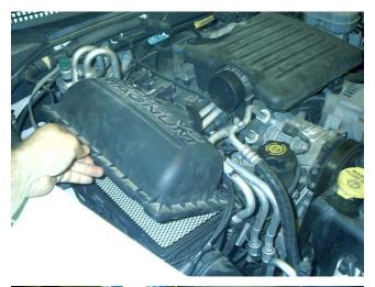
There are three clips holding the air box cover in place (two along the side and one on the back). Release these clips, and then lift up on the airbox cover as shown in the picture.
