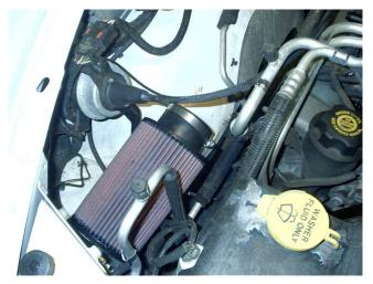
Set the filter in place on the fender well. The filter pictured is the one that comes with the manual transmission intake. The filter for automatic equipped vehicles is slightly smaller.
