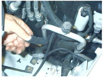
If you have a manual transmission, your intake kit included a piece of split rubber tubing. If your truck is equipped with air conditioning, slip it onto the A/C line as shown. This will prevent the filter from chafing the line in the event that they come into contact.
