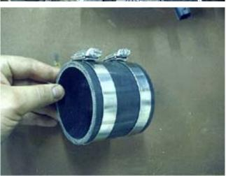
Note: Earlier versions of this kit have a two piece silicone connector which consists of a 3" ID x 1.5" section which fits inside of a 3.25" ID x 3" piece. This is used because the earlier tubes have a constant outside diameter of 3", and this size must be adapted to fit onto the 3.25" plenum.
