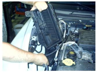
Removing the airbox from the engine will probably take some wiggling and maneuvering, but you should be able to remove it like so...
