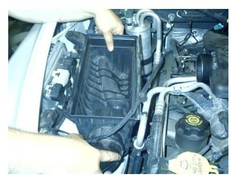
Next, grab the entire airbox unit and firmly pull up. It looks like there are two nuts at the bottom of the airbox, but they're really just push-on fasteners, and will release the airbox when you pull.
