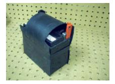
sections of the cover; one is about 6" long, and the other is slightly less than 5" long. The longer section should be at the back of the battery, covering the flat head screws and coming part way up the brackets. The narrow section of the cover goes over the
