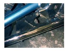
Use a Phillips head screwdriver to disconnect the negative and then the positive cables from the stock battery. Remove the two bolts from the lower front sides of the battery box using a 10mm socket or wrench, as shown at left. The bottom of the box will open, allowing the battery to be dropped down (gently!) and slid out from under the right side of the bike.
