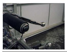
Next, either fold the remainder of the rubber strip up into the handlebar, or trim off the excess. *IMPORTANT:* Be sure to leave enough rubber so that you can grab it, either with your fingers or a pair of pliers. If you don't have enough rubber to grab onto, removing the weight will be VERY difficult!
