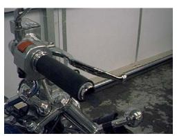
Once the cap has been removed, insert the strip of rubber so that approximately 1 to 1½ inches of the rubber is sticking out of the end. The rubber strips that are included have been purposely made "too wide". This is to allow for variations between handlebars. You will need to use a pair of scissors or a razor blade to make the strip thinner. (More on this later...)
