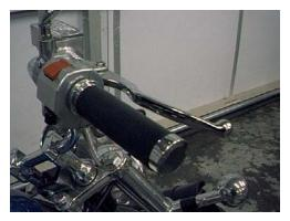
To the left is what we're starting with; a stock Suzuki Intruder handlebar. The first step is to remove the plastic "chrome" cap at the end of the grip. You should be able to simply pry it off with your fingers, though careful use of a screwdriver might be required if its stuck.
