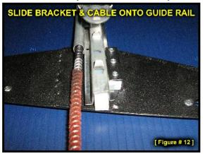
Slide the broken plastic bracket off the guide rail and install the replacement metal bracket as shown in *Figure 12*. The cable rides in the round channel, the nylon block in the middle of the bracket rides in the square channel and the nylon slot rides on the edge of the guide rail.
