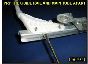
a number of ribs cast into it but the other side has none. Lay the main tube on your workbench such that the ribs are against the surface of the bench (facing down) and then press down on the rivet with your punch. The side of the main tube that is facing up in *Figure 9* should be facing down while you press the rivet through.)
