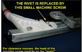
For clearance reasons, the head of the machine screw must be on the "metal" side of the guide rail, with the nut & lock washer on the "plastic" side, as seen here. [Figure # 13]
